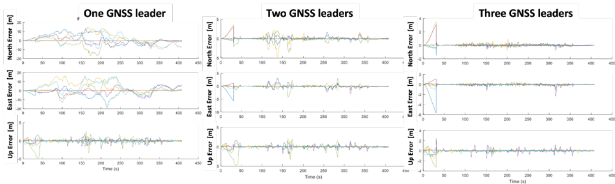
Figure 7-4: Filter results (errors) when one or more leaders have knowledge of the global (absolute) position due to their advanced equipment or advantageous location.
